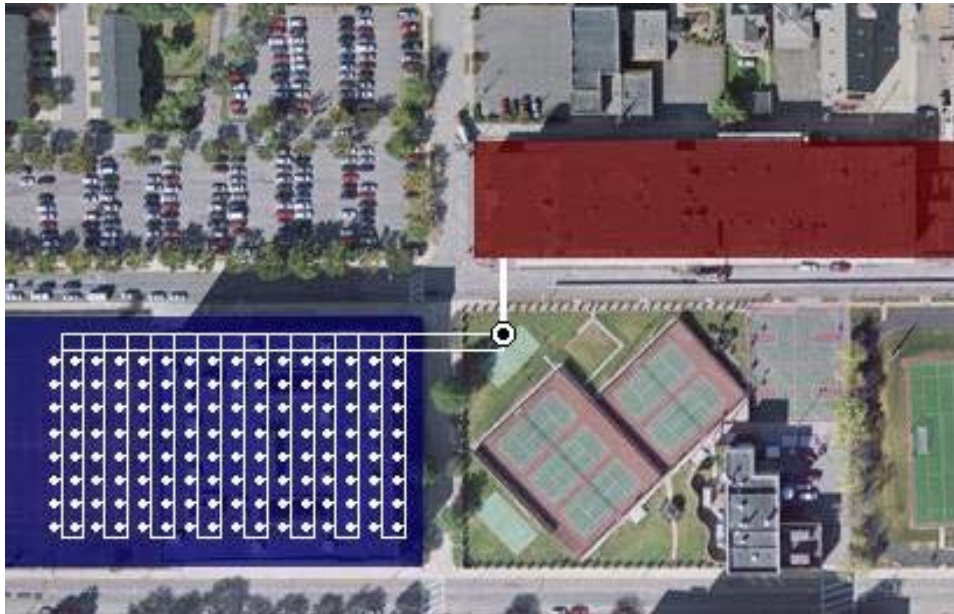
Figure 2-P. A visual depiction of the 8x16 loop field arrangement and its relation to the school.
